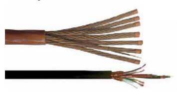
When moving a cable electrostatic charges and voltages occur due to internal friction. As these voltages, called "microphony", may have up to 0.5 V, the actual measured signal will be blotted out. Low noise measuring cables are designed to emit extremely low microphony voltages, in specially constructed cables the microphony voltage is even below 0.1 mV. The quality of the potential balancing layer is essential for this advantage in the measuring technology.
